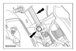
16. Mark the position of the 4 subframe nuts and 4 subframe bolts for referencing during assembly.
