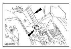
8. NOTE: Do not tighten the subframe nuts and bolts at this time.
