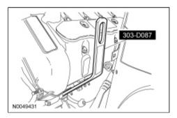
9. Install the Engine Lifting Bracket.
